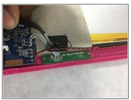
Using tweezers, carefully remove the tape that is holding the black and red intertwined cables to the motherboard. Place tape to the side as it will be needed for reassembly.
