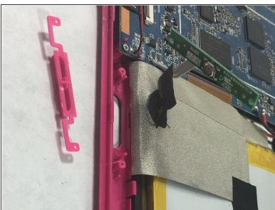
Using tweezers, slowly and carefully remove the end of the cable that connects the home button to the main motherboard.
