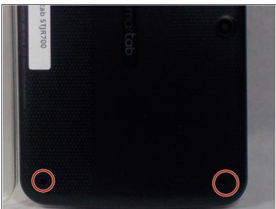
Power off device. Place it face down. Unscrew the four perimeter screws using a PH000.
