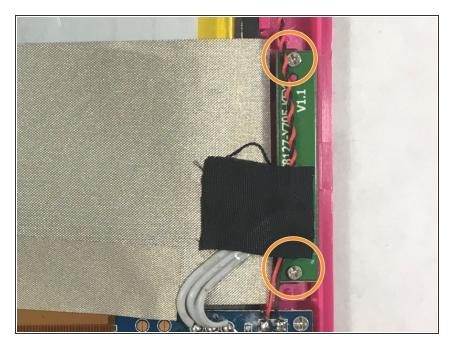
Remove the two Phillips #000 screws holding the home button board to the front panel.
