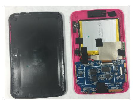
Using a plastic opening tool or metal spudger, begin to gently pry the rear case down and away from the display. Slowly wiggle the tool up and down to pry open the tablet.
