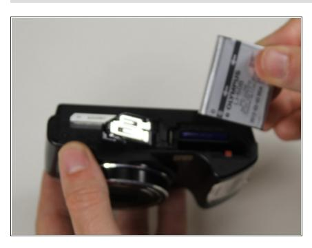
Remove the battery from the battery compartment.
