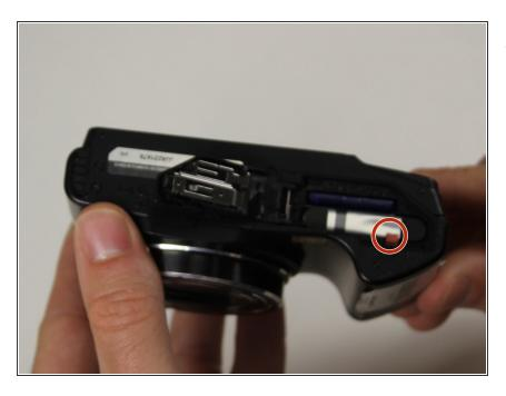
Push down on the red retaining button to release the battery.
