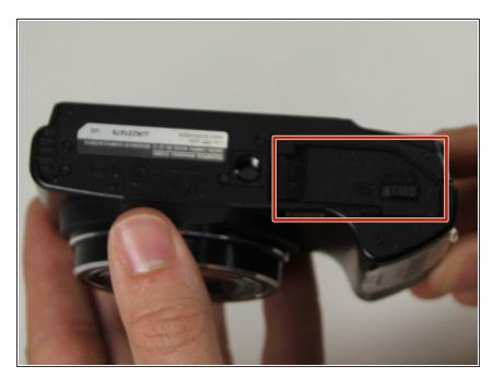
Slide the small, textured tab on the bottom of the camera to open the battery compartment.
