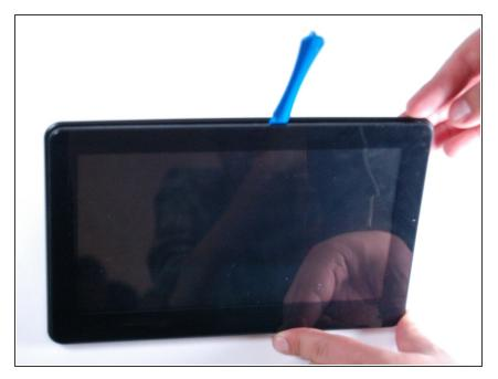
• First, you will need to open up the tablet using the wedger.
