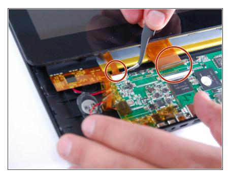
• Carefully remove the touch screen tape sensors using tweezers in order to separate the two halves.
