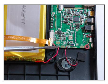
• You will need to desolder the battery from the motherboard. Once its off you just solder the new battery in its place.
