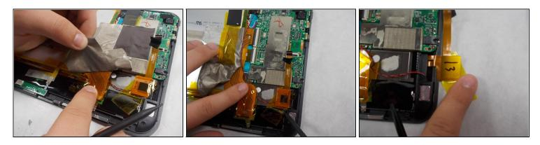
• Peel up the grey tape so that you can get to the board and untape the ribbon cable that was removed from the motherboard in the previous step.
