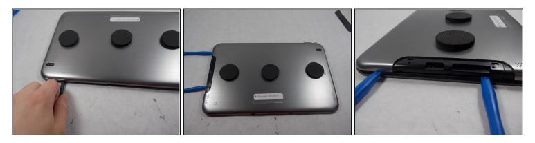
• Pry around the outside carefully using the black spudger to get in. Putting many opening tools around the edge helps keep it from sealing shut again.
