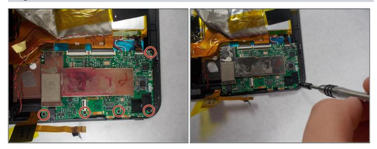
• Remove the two 1.2mm screws from the board.
