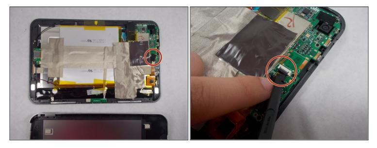
• Remove the ribbon cable by using the black spudger to release the tab and carefully pull out the ribbon cable.
