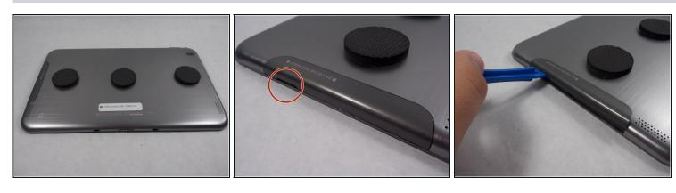
• Use an opening tool to pry off the memory card door located on the back of the tablet.
