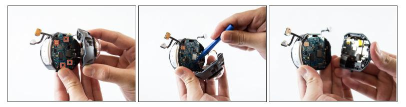
Insert a plastic removal tool underneath the four sensors on the motherboard to fully separate the camera case.
