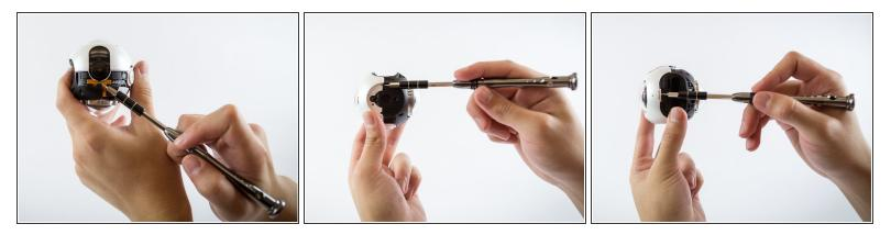
• To remove the left cover of the camera body, lift the left cover using a small flathead screwdriver and pull it off.
