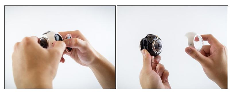
• Using both hands, carefully remove the right cover off the camera body.
