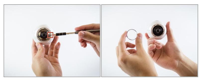
• Insert a small flathead screwdriver into marked slot on camera lens and pry off camera lens cover.
