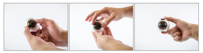
• Twist silver ring on the lens counter-clockwise with force to remove it.
