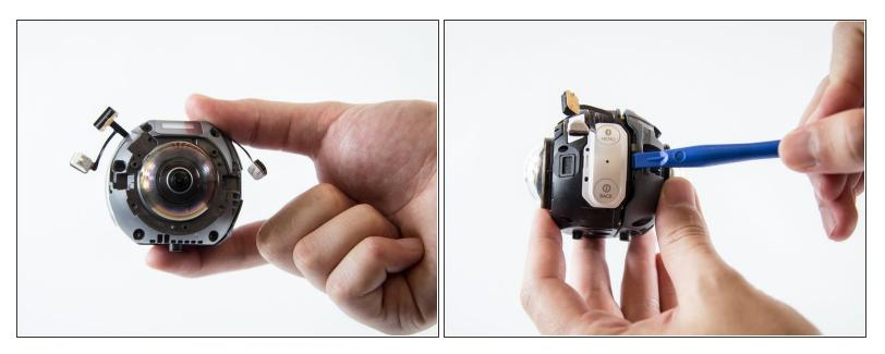
• Carefully use a plastic opening tool to separate the gray case from the black case on the device.
