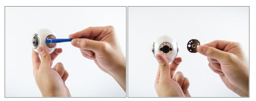
• Using a plastic opening tool, pry the tripod mount off the device.
