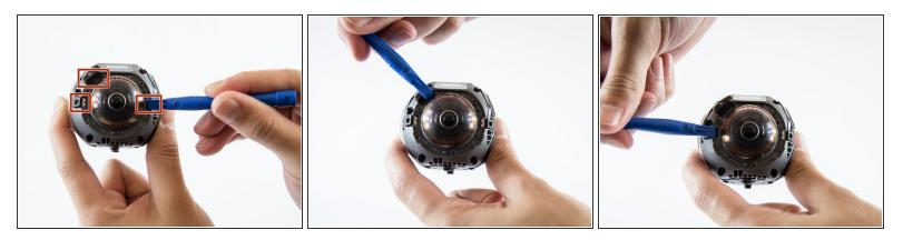
• Carefully lift the three sensors off using a plastic opening tool and pull them aside.
