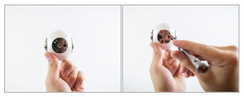
Once the black rubber has been removed, unscrew all Phillips #00 0.75 mm screws on the bottom of the device using a PH00 screwdriver head.
