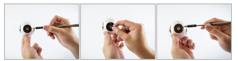
Peel off the black rubber located on the bottom of the device using your hand or a small flathead screwdriver.
