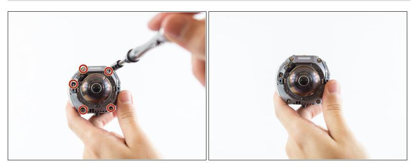
Remove all Phillips #00 0.75 mm screws from the body of the camera using a PH00 screwdriver head.
