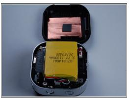
Pop open the back cover of the camera battery using a plastic opening tool.
