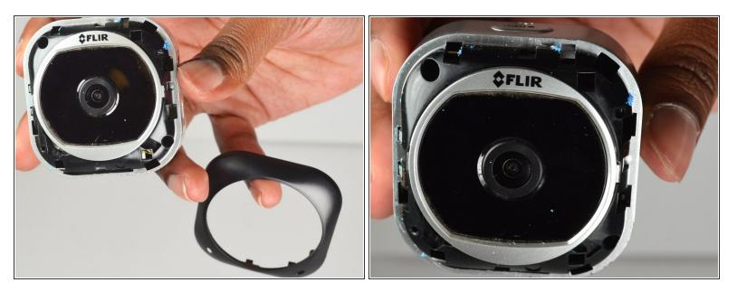
• Pop off the black covering so the square camera lens is completely exposed.
