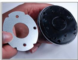
Once you have separated the two parts, use a J00 screwdriver to unscrew the four 1.2 mm screws which connect the metal piece to the top of the the stand.
