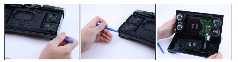
• Pry off and separate the black plastic casing.
