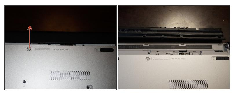
Remove the battery. Pull the battery forward and remove it from the laptop.
