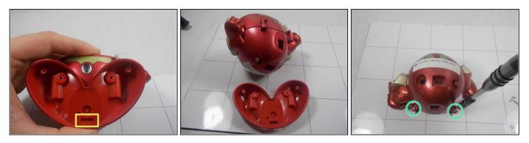
• Use a spudger to release the small retaining clip that holds the feet to the bottom of the device.
