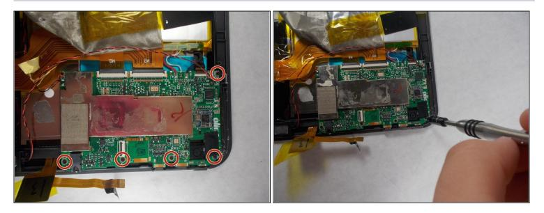
Remove the five 1.2mm screws from the board.
