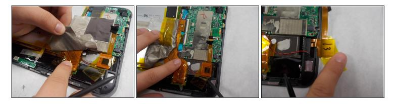
Peel up the grey tape so that you can get to the board and untape the ribbon cable that was removed from the motherboard in the previous step.
