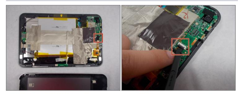
Remove the ribbon cable by using the black spudger to release the tab and carefully pull out the ribbon cable.
