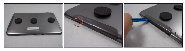
• Use an opening tool to pry off the memory card door located on the back of the tablet.
