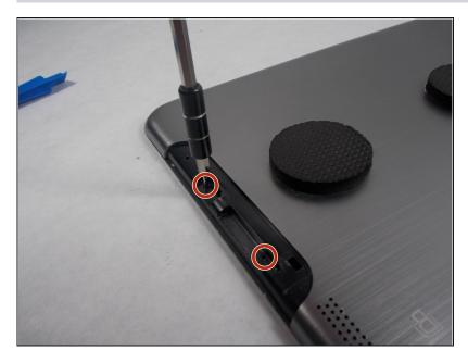
Remove the two 1.2mm screws found under the memory card door.
