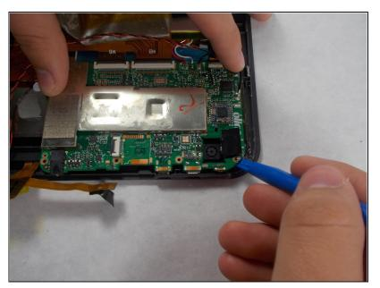
Use an opening tool to remove the board from the case.
