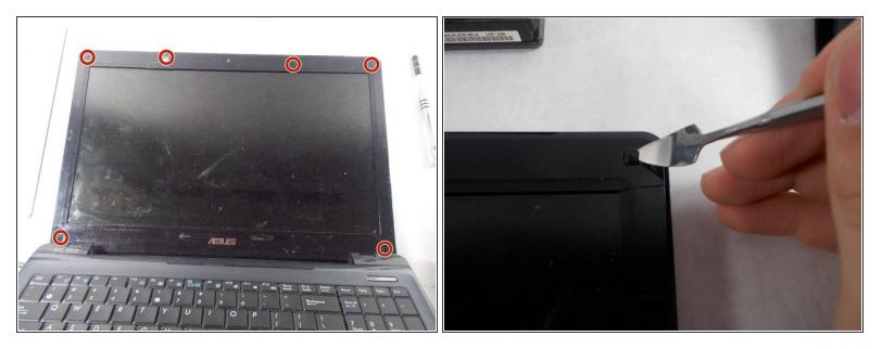
• Remove the six rubber pads around the border of the screen using a spudger.
