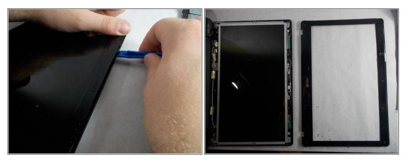
• Separate the plastic bezel from the rest of the screen using an opening tool.
