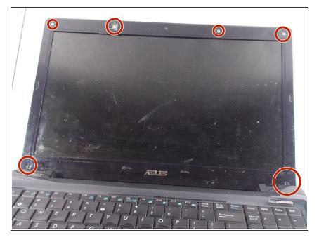
Remove the six screws using a Phillips #0 screwdriver.
