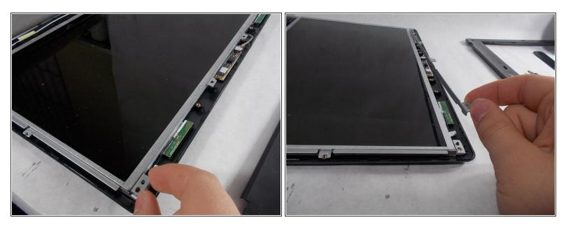
• Lift the metal bar on the top of the screen away from the device.
