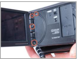
• Use the Phillips #00 head to remove the following 5.5mm screws on the left-hand side.
