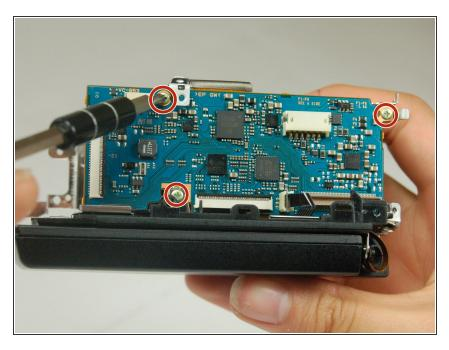
Use the Phillips #00 head to remove the following 5.5mm screws from the side of the motherboard.
