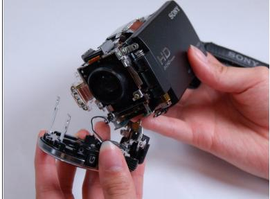
Carefully pull the lens cover and shutter assembly off of the front of the camera.
