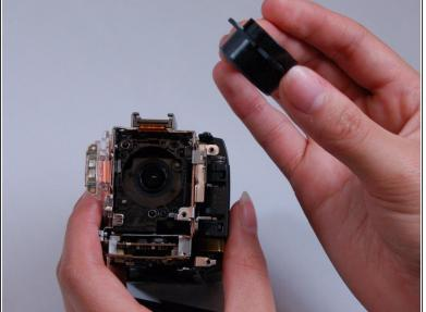
Carefully remove the lens from the body of the camera.
