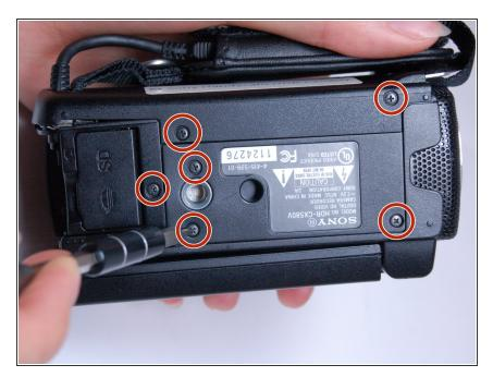
Use the Phillips #00 head to remove the following 5.5mm screws on the bottom.
