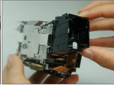
Use the Phillips #00 head to remove the following 5.5mm screws and remove the lens compartment by carefully pulling it out of the metal casing.
