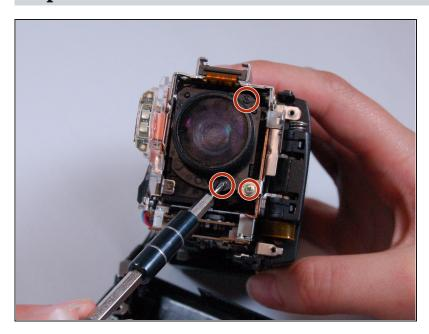
• Use the Phillips #00 head to remove the following 5.5mm screws on the lens shell.
