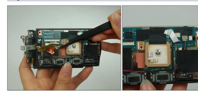
• Carefully use the <u>tweezers</u> to detach the following ribbon cable connectors.
