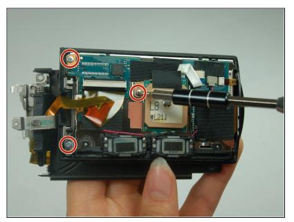
Use the Phillips #00 head to remove the following 5.5mm screws underneath the back casing of the screen.
