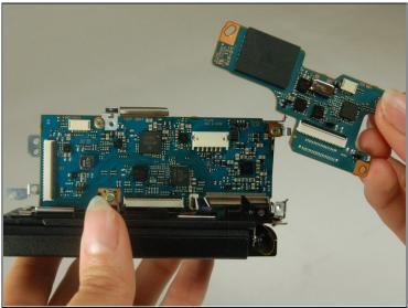
• The camcorder's chip and part of the motherboard should naturally fall off at this point and should carefully be removed and placed to the side.
