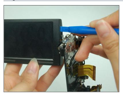
Use the plastic opener tool to loosen the casing between the screen's front and back.
