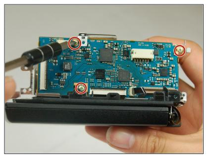
Use the Phillips #00 head to remove the following 5.5mm screws from the side of the motherboard.
