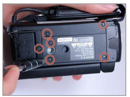
Use the Phillips #00 head to remove the following 5.5mm screws on the bottom.
