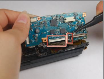
• Using a pair of tweezers, remove the following ribbon cable connectors to remove the motherboard from the camcorder.
