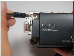
• To begin removing the metal casing, use the Phillips #00 head to remove the following 5.5mm screws.
