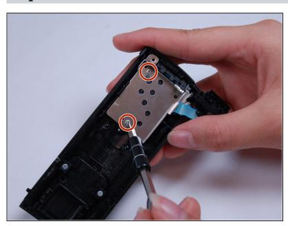
Use the Phillips #00 head to remove the following 5.5mm screws on the inside of the top casing.
