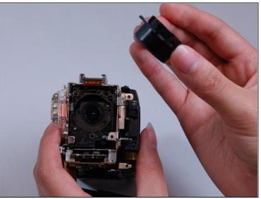
• Carefully remove the lens from the body of the camera.
