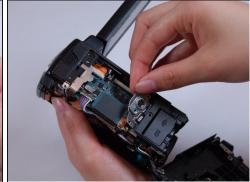
• Carefully remove the bottom casing with your fingers.
