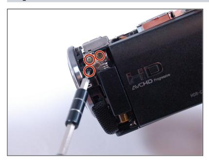
Use the Phillips #00 head to remove the following 5.5mm screws underneath the casing strip.
