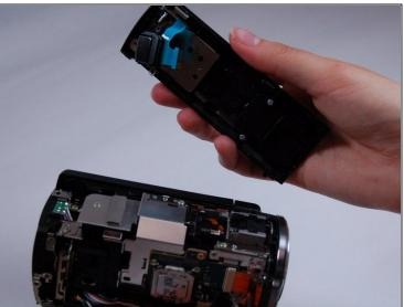
• Pull off the top casing by lightly grabbing either side and pulling towards the back of the camera.
