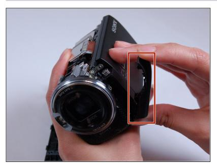
Carefully pop off the casing strip on the camera's left-hand side near the lens.
