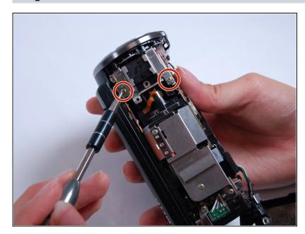
Use the Phillips #00 head to remove the following 5.5mm screws on the top near the lens.
