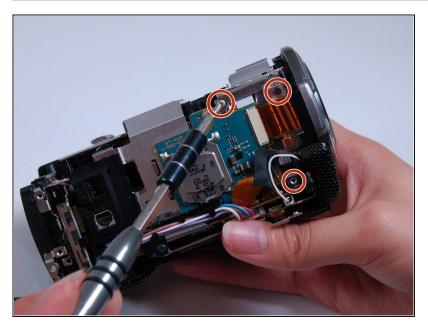
Use the Phillips #00 head to remove the following 5.5mm screws on the right-hand side near the lens.
