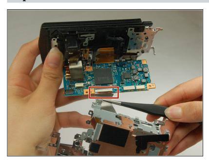
Using a pair of tweezers, remove the ribbon cable connector attached to the metal casing and the motherboard.
