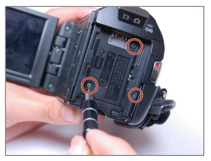
Use the Phillips #00 head to remove the following 5.5mm screws on the empty battery socket.
