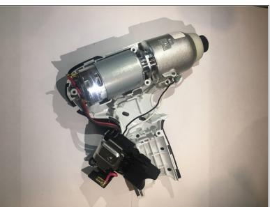
Place the big trigger out to be able to remove the other trigger smoothly.
