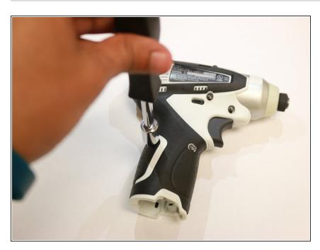
Unscrew the six screws on the top of the drill.
