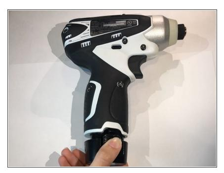
Place your fingers on the grip to pull out the battery from the device.
