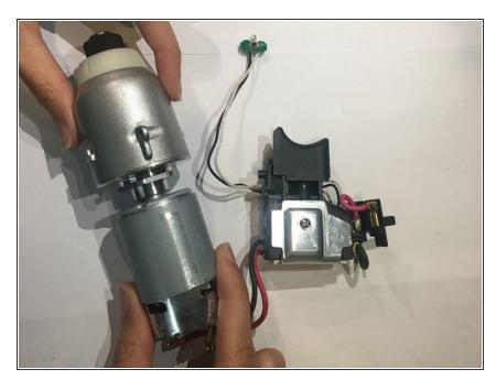
Pull both ends of the device to separate the motor from the rest of the device.
