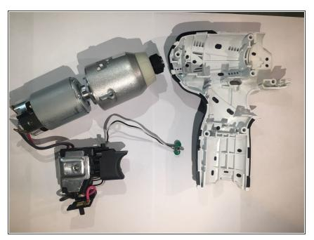
• Remove the bottom of the plastic drill case
