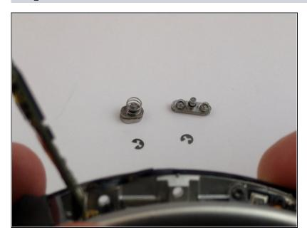
Remove the buttons, being careful not to lose the springs.
