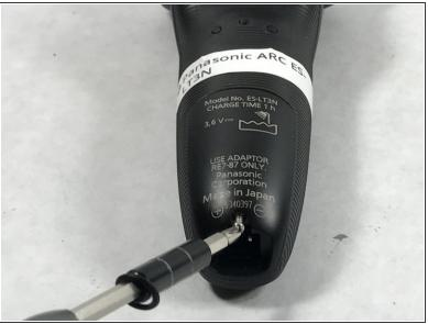
Using a Phillips #00 screwdriver, remove the 6 mm screw just above the charger port.
