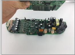
Lift control board up and away from power supply board
