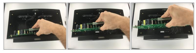
Remove circuit board by lifting it straight away from the rear plate.
