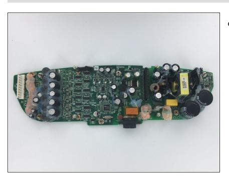
The larger of the two boards is the power supply board.
