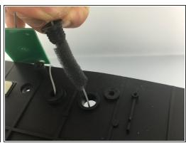
Remove second rubber strain relief by pinching the rubber then lifting up and away.
