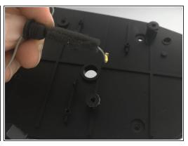
Remove first rubber strain relief by pinching the rubber then lifting up and away.
