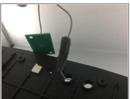
Remove third rubber strain relief by pinching the rubber then lifting up and away.
