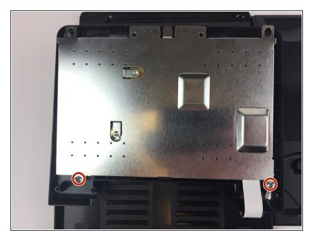
• Place the video screen face down to expose the two screws. The screws are indicated by the red circles.
