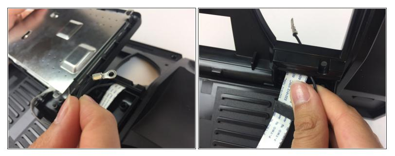
Pull the ribbon connector and blade connector through the top case.
