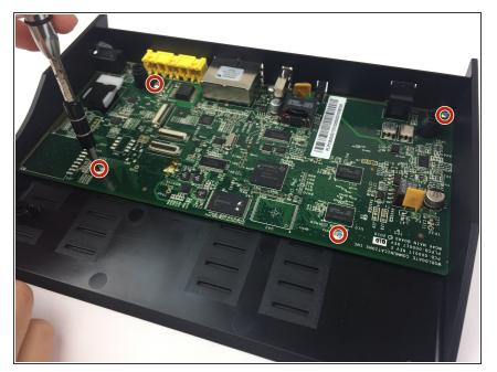
Use the Phillips #0 Screwdriver to remove the four Phillips head screws (6 mm) highlighted by the red circles.
