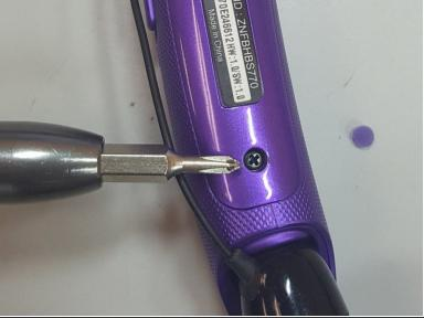
Remove both of the hidden screws using a Philips #00 screwdriver.
