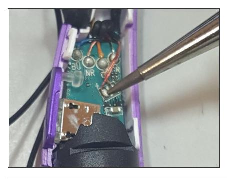
Desolder speaker connection from board using a solder iron.
