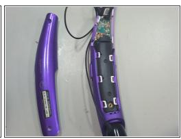
Use a guitar pick or any pry opening tool to open the housing.
