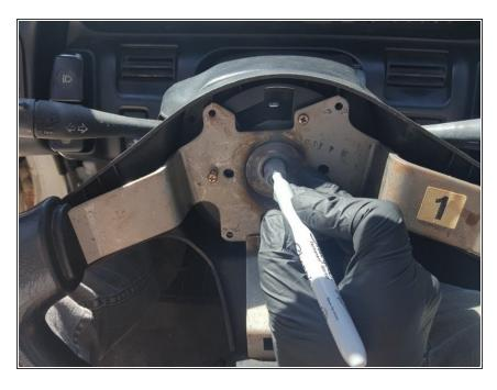
Use a paint marker to mark a reference point for the top center of the steering wheel on the face of the steering shaft.
