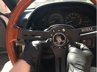
Press the horn into the inner horn retainer.
