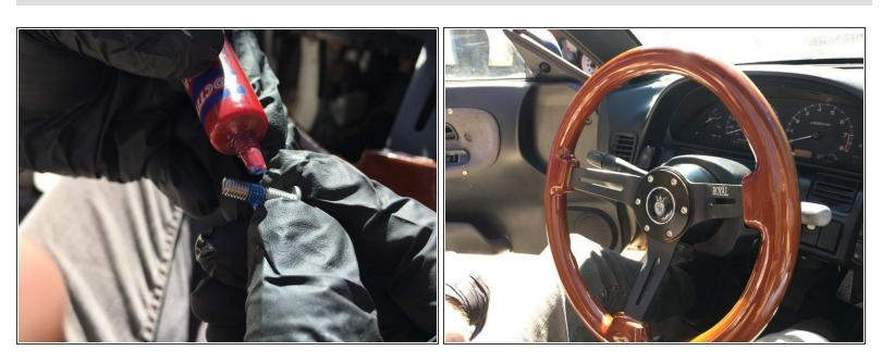
Place a drop of low strength thread locking compound to each screw and thread them into the steering wheel hub.
