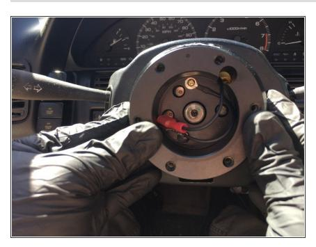
Install the steering wheel hub onto the steering shaft, aligning the top center mark on the hub with the paint mark you made in Step 4.
