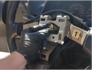
Using a 19mm socket and ratchet, loosen the steering wheel retainer nut and remove it.
