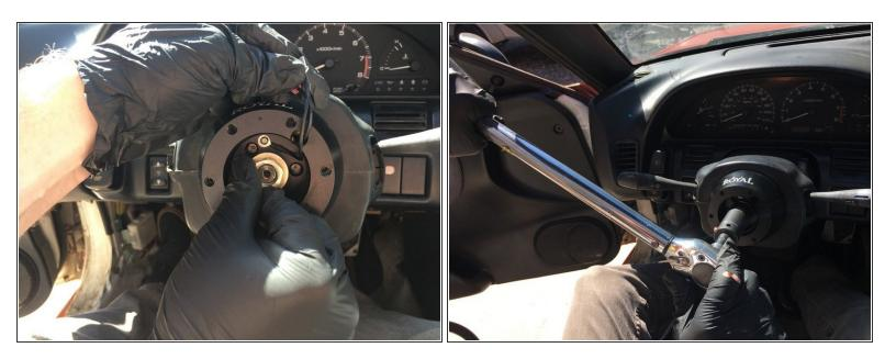
Reinstall the steering wheel retaining nut torqueing it down to 29 ft\*lb using a torque wrench.
