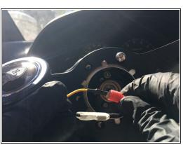
Make the wiring connections for the horn.
