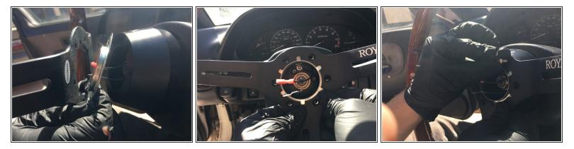
• Place the inner horn retainer ring in-between the new steering wheel and hub, aligning the six bolt holes, and place one screw, finger tight, in the hub to temporarily hold everything in place.
