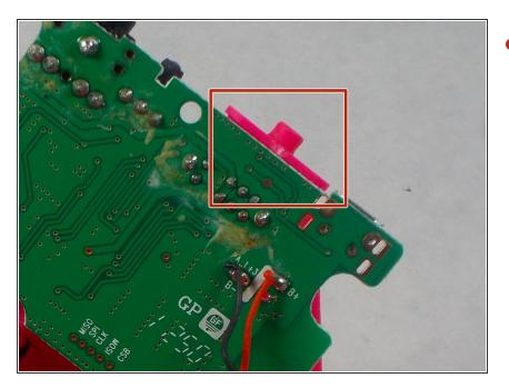
Remove the plastic cover from the power switch actuator on the motherboard.
