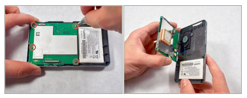
• Using a screw driver, unscrew the four 2mm screws holding the motherboard in place.
