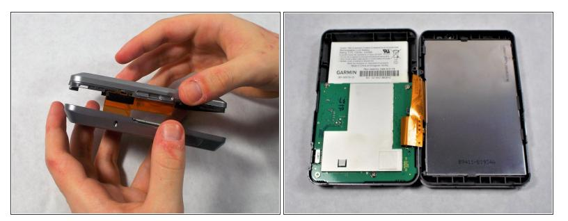
After the case front and rear are separated, carefully lay the two sides down without disconnecting or damaging the orange ribbon cable.
