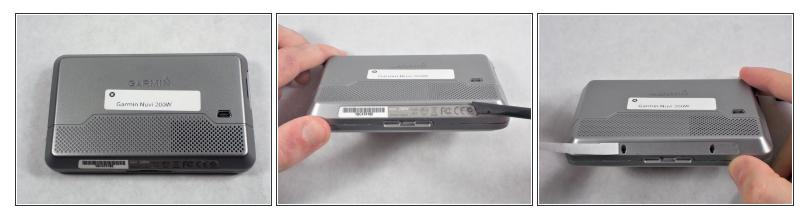
• Peel off the sticker in order to find the two Torx T5 screws.
