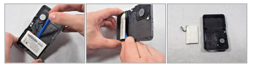
Using your opening tools, separate the battery from the top side. Very slowly push your tool down into the crevice.
