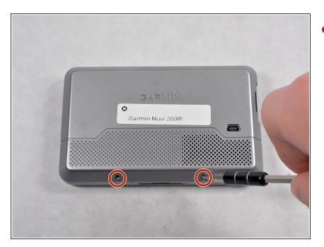
Remove the two 4mm T5 Torx screws.
