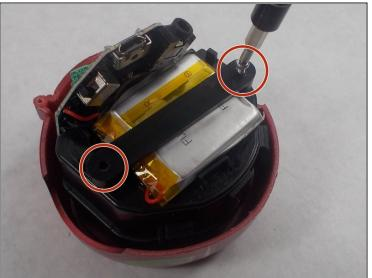
• Loosen and remove the two Phillips screws holding down the battery cover (the black plastic strip that keeps the battery in place).
