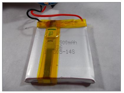
Gently lift the battery from the rest of the front assembly to stretch the wires out slightly.
