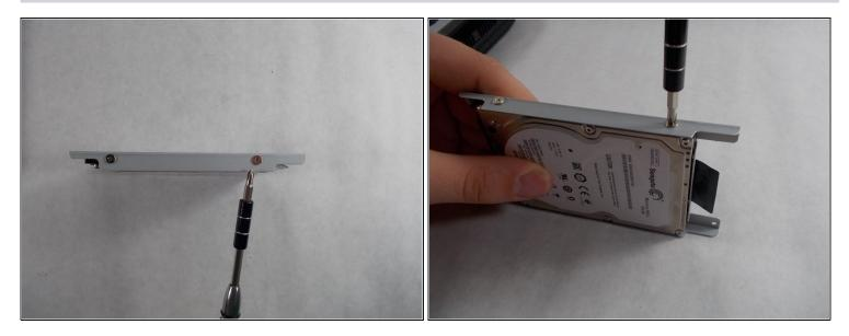
• Using a Phillips #0 screwdriver, remove the cage screws on the side of the hard drive.
