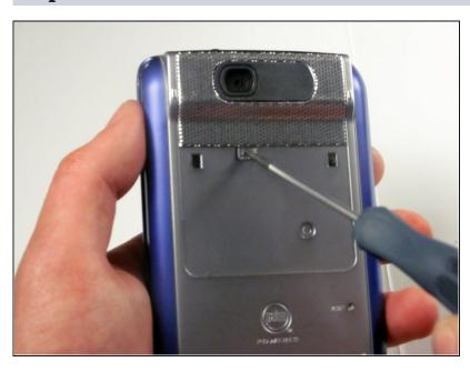
Use a #00 Phillips screwdriver to remove the 2.5 mm hidden screw.
