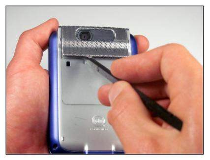
Use either end of the spudger to carefully pry off the camera lens mesh cover.
