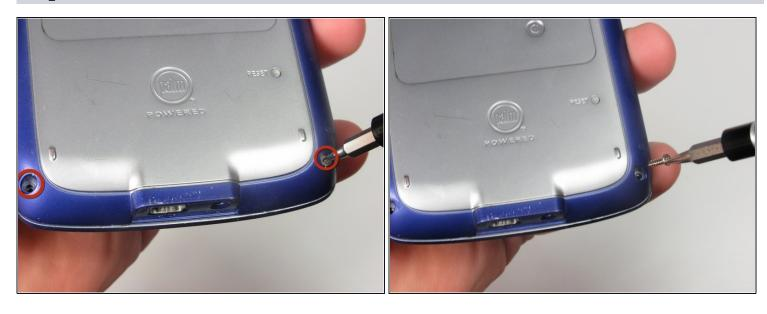
• Using a T5 Torx screwdriver, unscrew the two 5mm screws located at the bottom of the device.
