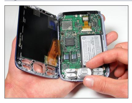
Remove the control pad buttons from the device and set aside.
