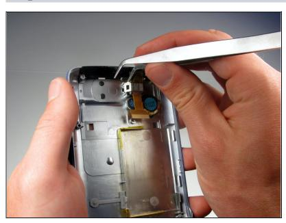
• Using <u>tweezers</u>, pry one side of the clip off.
