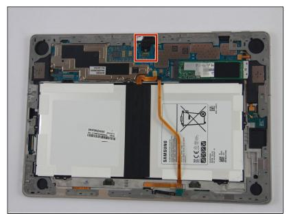
Locate the camera and its corresponding connecting port.
