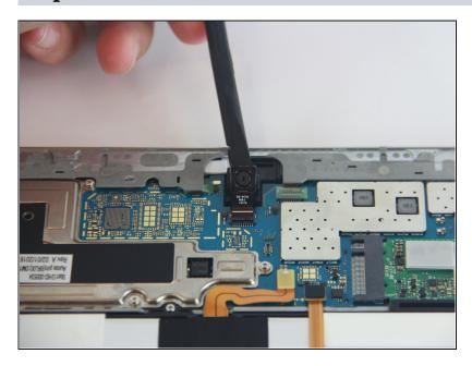
Proceed to lift up the camera out of its resting position.
