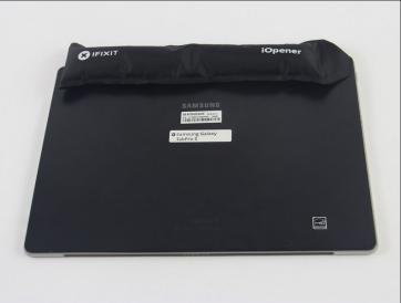
• Heat the iOpener in the microwave for 30 seconds. Then place it on each side for 20 seconds in order to loosen the adhesive sealing on the device.
