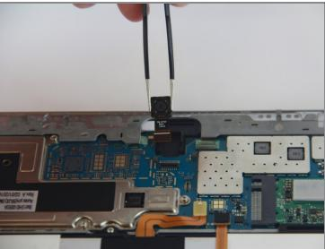
• Simply pull the camera parallel to the device out of its connecting port.
