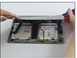
• Using the plastic spudger, open up the back of the device.
