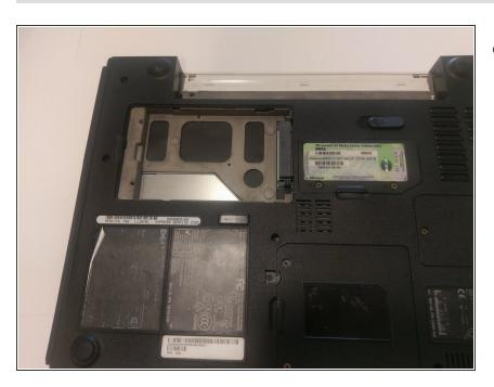
Remove the old HDD from the casing. This is done by simply sliding it out.
