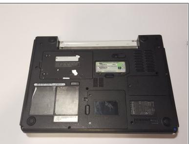
Slide the lock and pull out the battery.
