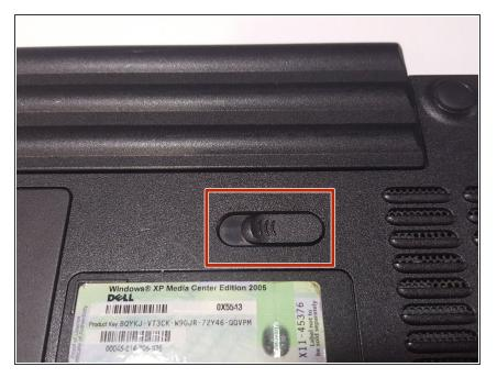
Locate the slide lock for the battery.
