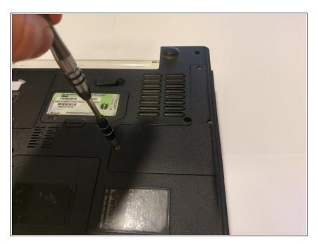
Unscrew all screws that hold the cooling module cover in place
