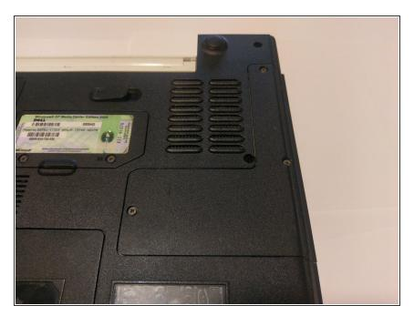
Locate cooling module cover on the underside of the laptop
