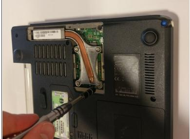
Unscrew the screws holding the metal bracket in place
