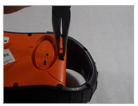
Remove the 15 rubber plugs from the cavities using needle nose pliers.
