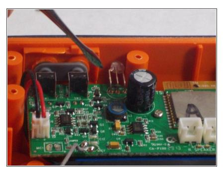
Insert the new LED light into the frame. Use the solder and soldering iron to reconnect the terminals to the new lights.
