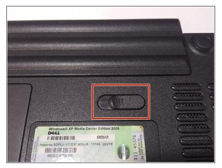
Locate the slide lock for the battery.
