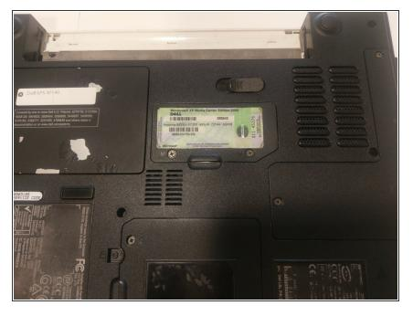
Locate RAM carriage on the bottom of the laptop
