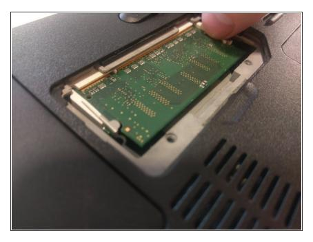
Squeeze clips that hold the RAM card in place
