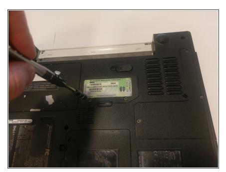
Unscrew both screws holding the cover in place
