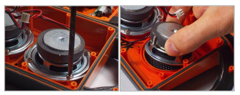
• Remove the four screws that hold down the speaker and pry up the speaker from the frame.
