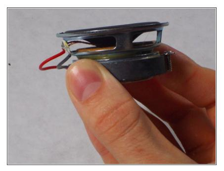
Once the voice coil is removed, solder it back onto the bracket or replace the voice coil entirely.
