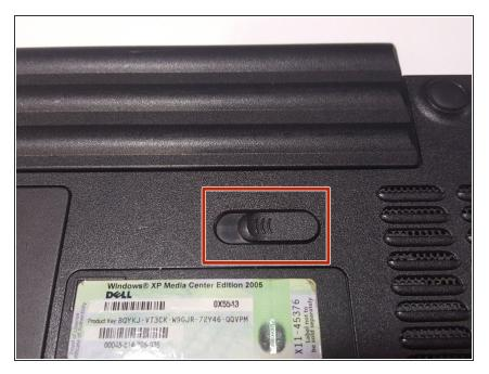
Locate the slide lock for the battery.
