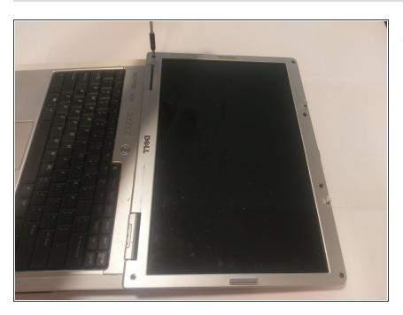
Unscrew the screws on the casing that you just exposed.
