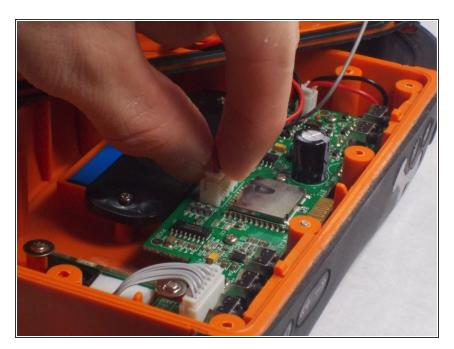
Disconnect the wiring to improve accessibility to the battery.
