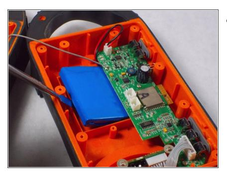
Pry the battery from the frame using your hands or an opening pick.
