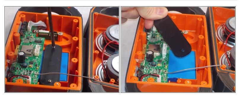
Remove the two screws that hold that bracket, securing the battery in place.
