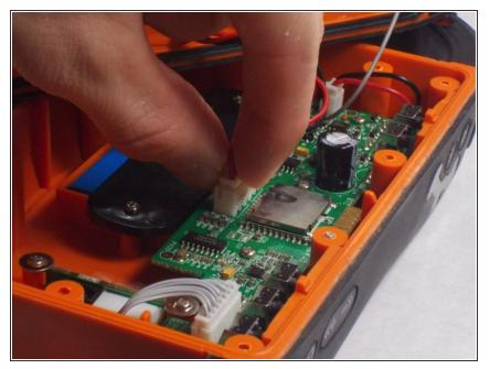
• Disconnect the wiring to improve accessibility to the cones.
