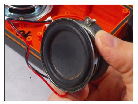
• To replace the cone, remove the existing one by peeling it off of the speaker with needle nose pliers.
