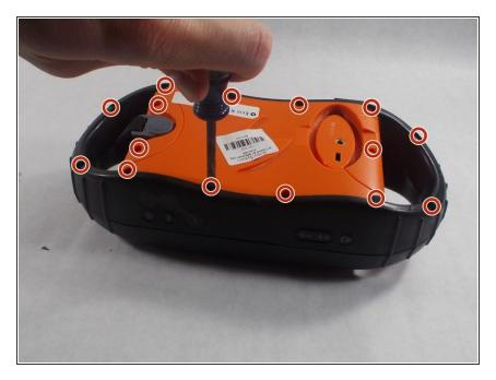
• Use a phillips head screwdriver to remove the fifteen 6.4mm screws.
