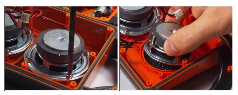
• Remove the four screws which hold down the speaker. Then, pry up the speaker from the frame.
