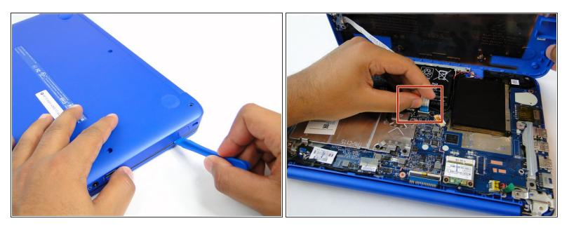
After removing all the screws, slowly and carefully lift the back cover, exposing the internal components.
