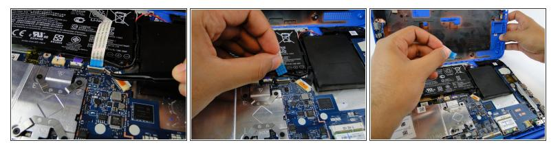
• Carefully detach the blue strip that connects the back cover to the internals.
