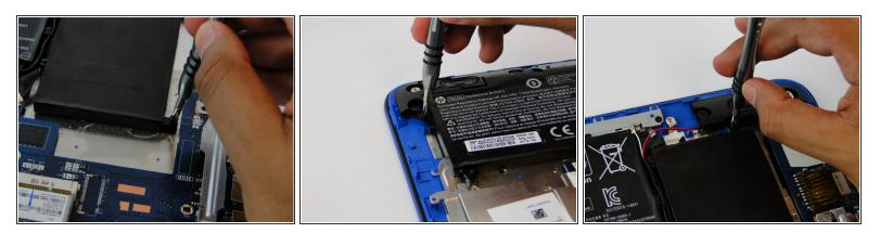
• Using the JIS J0 screwdriver, unscrew the 6.5 mm screws surrounding the battery.
