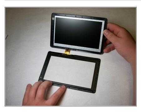
Once the glass and display have been separated, pull the glass away from the display and carefully slide the ribbon cable out of the display housing.
