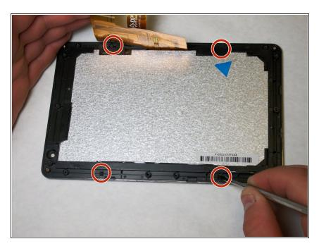
Using the metal spudger, depress the four plastic tabs to free the glass from the display.
