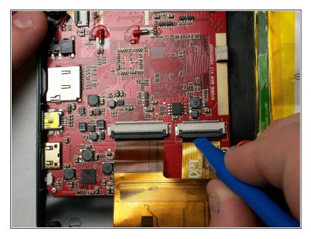
Using the plastic spudger, lift the black latches for the ribbon cables and slide the cables out of their sockets. Now the two halves can be separated.
