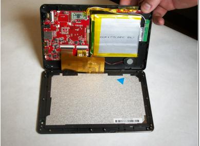
Separate the back from the screen and open as shown. Make sure to open from the side with the power button to avoid damaging the ribbon cables.
