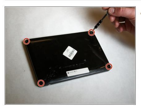
Remove four Phillips head screws from back with #0 screw driver.
