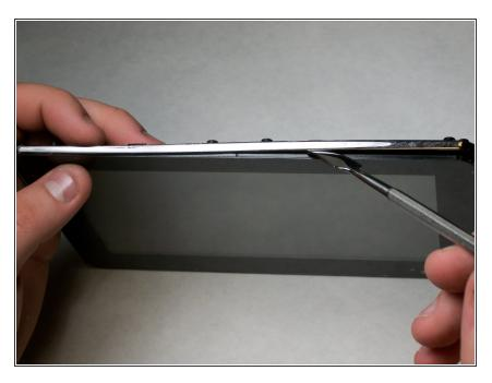
Use the metal spudger again to get between the glass and the chrome trim ring. Lightly pry the glass away from the display. If this proves difficult, double check that all of the screws have been removed and that all four plastic clips are pushed in. Again, start from the side opposite the ribbon cable to avoid damaging it.
