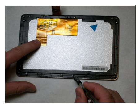
There are 14 3mm long screws surrounding the screen. Using the #00 Phillips screwdriver, remove all of these screws.
