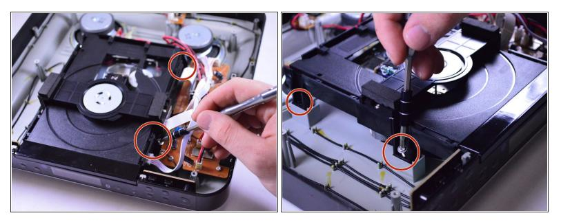
• Remove all four screws(13.5 mm in length) that are securing the disk drive.
