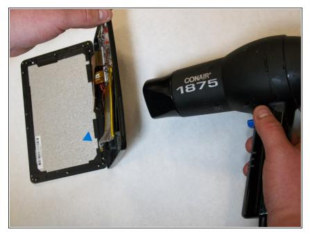
• Heat up the back of the device with a hair dryer to loosen the glue.
