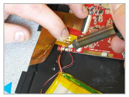
• Desolder the two battery cables from the mother board.
