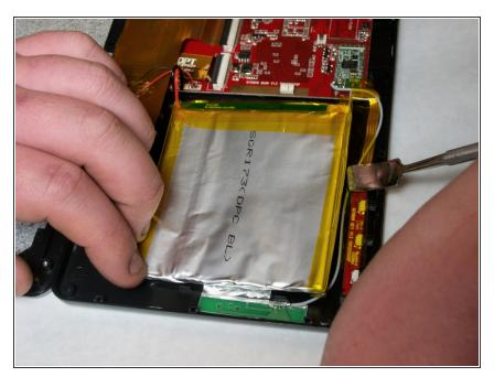
Pry up battery from plastic using a nylon spudger or plastic opening tool.
