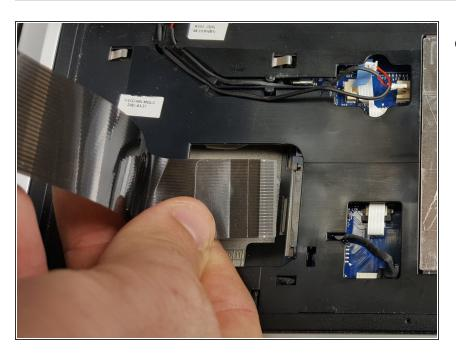
Lift up on the keyboard and remove ribbon from its connector.
