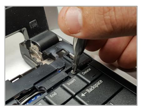
Remove two 4.65mm screws on top of the keyboard.
