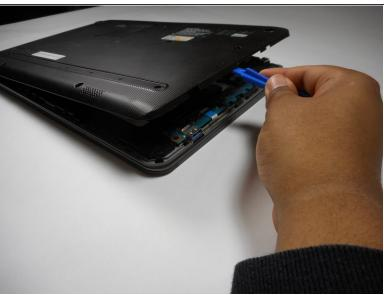
Remove the back panel open by inserting the plastic opening tool into the seam of the laptop and pushing downwards. Repeat the motion around the perimeter of the device.
