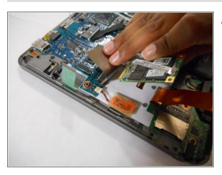
Completely remove the hard drive from the device.
