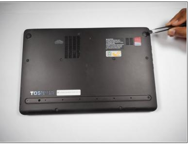
Use tweezers to pinch and pull out and remove the nine rubber gripper pads on the back panel of the laptop. Set aside.
