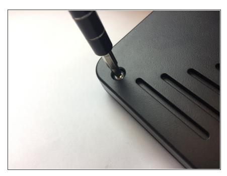
Use the Phillips #0 Screwdriver to remove the four Phillips head screws (6 mm).
