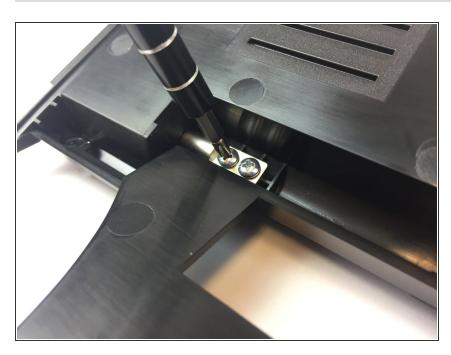
Use the Phillips #0 Screwdriver to remove the two Phillips head screws (5 mm) located on the upper case.
