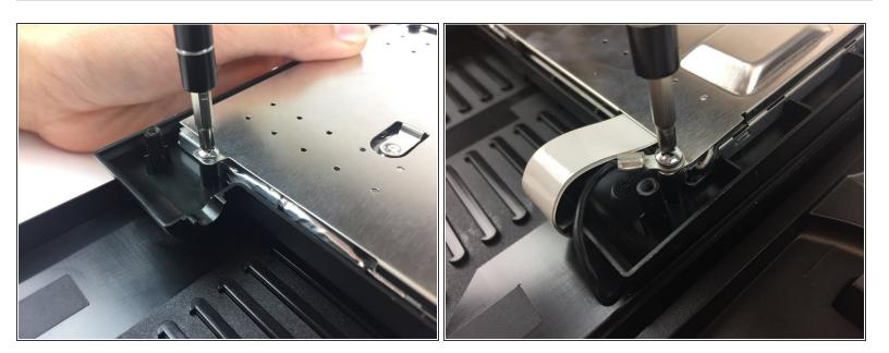
Use the Phillips #0 Screwdriver to remove the two Phillips head screws (6 mm)
