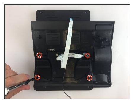
Use the Phillips #0 Screwdriver to remove the four Phillips head screws (6 mm) highlighted by the red circles.
