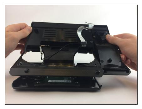
Gently lift up on the upper case to separate it from the keypad/speaker panel.
