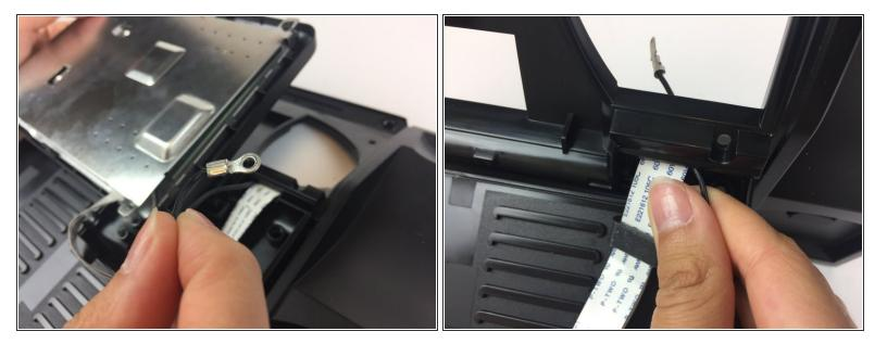
Pull the ribbon connector and blade connector through the top case.
