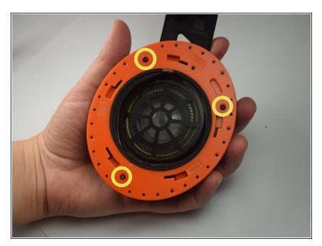
Using the Phillips #0 screwdriver, remove the 6.0 mm screws on the orange plate.
