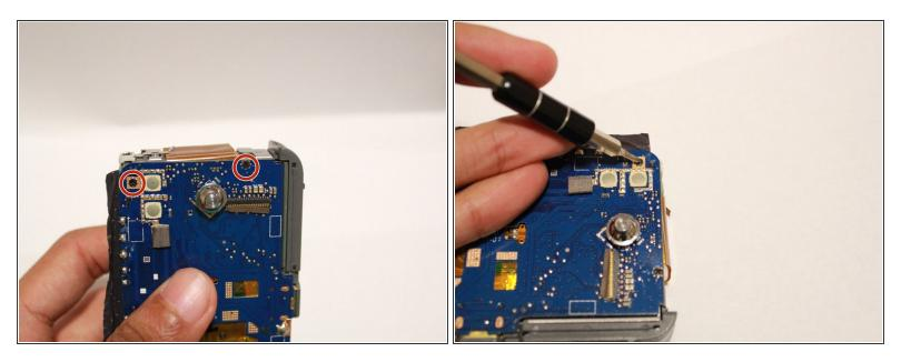
• Use a J00 screwdriver to remove two screws located on the far right, near to the main button.
