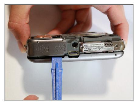
• Pull the outer case off using the plastic opening tool.
