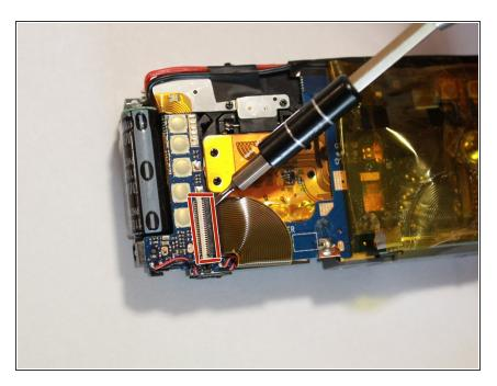
Unplug the connector by lifting the little lock holding it in place.
