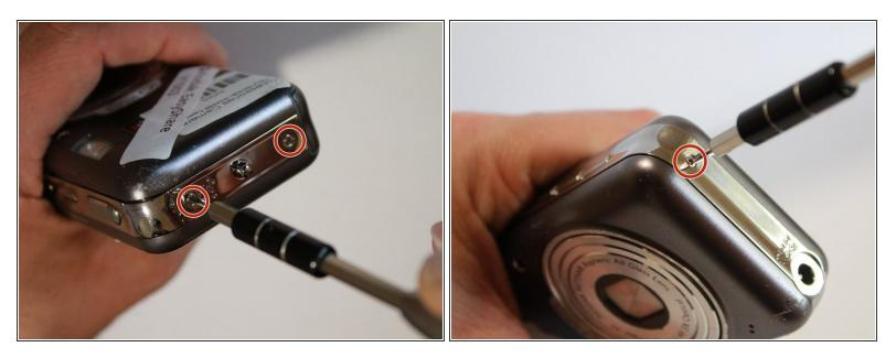
Use a J00 screwdriver to remove the five exterior screws.
